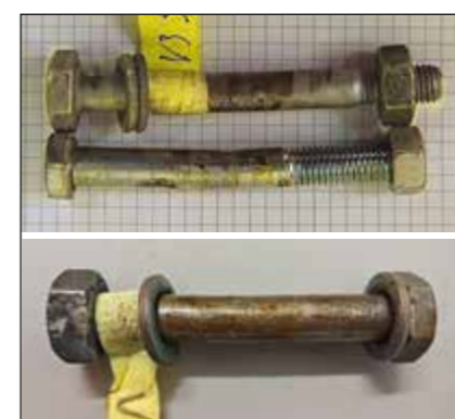
Fig. 3: AScrews removed from the test specimens after the explosion with diameters M12 (left) and M16 (right)
