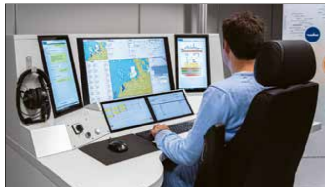
Fig. 1: Realisation of standard console with COTS hardware
