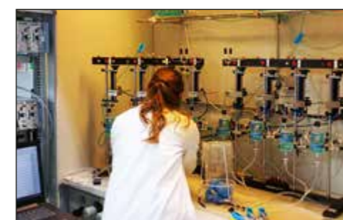
Fig. 5: Multi-organ bath with 12 myographs to examine the function of respiratory muscle preparations from different species. Investigation of new compounds on respiratory muscle poisoned by chemical agents
