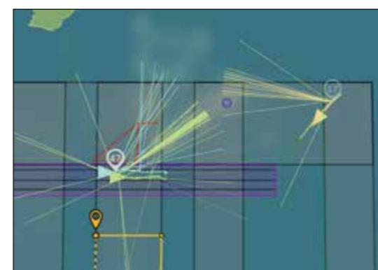
Fig. 3: Near-real time operational picture of glider position and tracks from 18 Sep 2024 along with associated bearings from detections throughout the day, all displayed in SeaSuite. All three gliders appeared to be detecting a target in the same area
