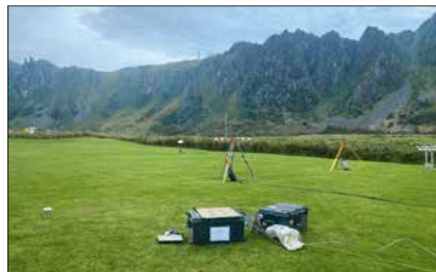
Fig. 1: Two ISL GNSS systems on the test range with the high-power jammers (on the top of the mountain side) at a distance of 1.5 km
