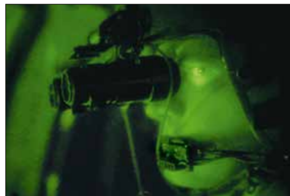
Fig. 1: NVGs are usually clipped on the pilot's helmet. The field of view is strongly limited (source: Wikimedia Commons)
