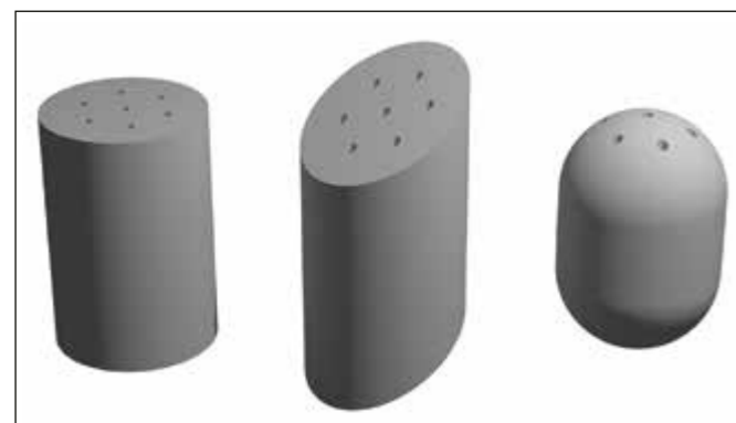
Fig. 1: CAD model of a conventionally manufactured cylindrical solid propellant with varying cutting angle (left, centre) and a solid propellant that cannot be manufactured conventionally (right)
