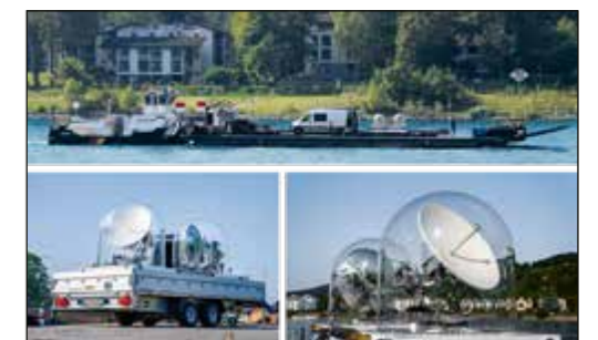
Fig. 4: SABBIA® system mounted on a moving ship
