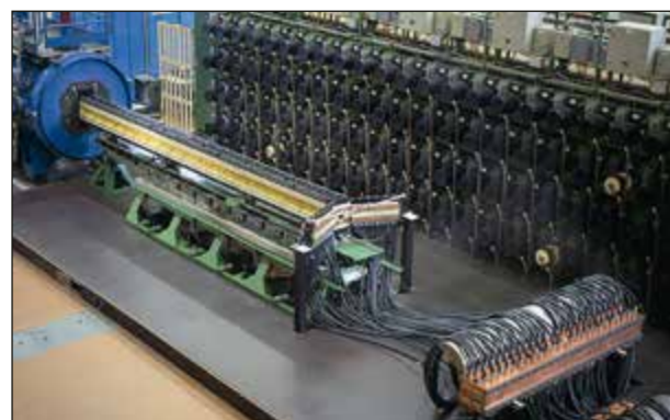
Fig. 1: NGL 60 railgun “PEGASUS” and capacitor-based power supply
