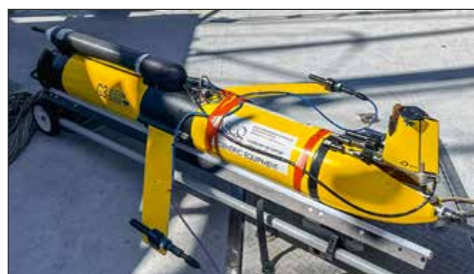
Fig. 2: Photograph of the two TWR gliders. For both of them, the OceanObserver acoustic recording system was built into an extra housing, mounted on top of the glider. As part of the data analysis, the pros and cons of the different configurations are being evaluated (with respect to flow drag, acoustic self-noise, ease of maintenance, etc.)
