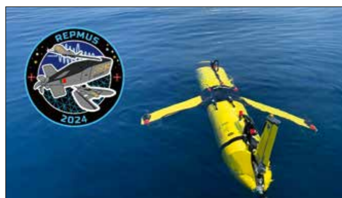
Fig. 1: A photo of WTD 71's Slocum glider taken during an in-sea swap of hydrophones. The acoustic recording system OceanObserver is integrated into this glider. The embedded image shows the official REPMUS 24 logo
