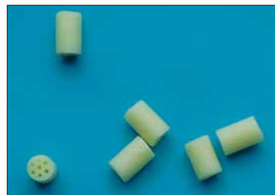
Fig. 1: Plastic-bonded gun propellants in cylindrical geometry with seven perforations for the evaluation of new materials and formulations with new and modern nitrate-based and azido plasticisers
