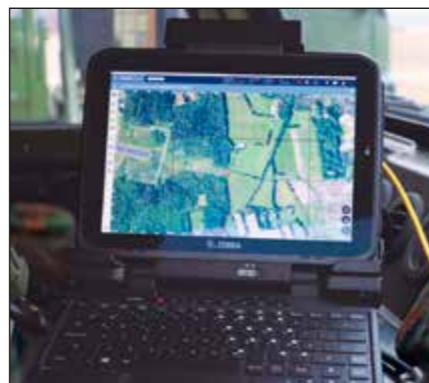
Fig. 2: Situational display SitaWare Frontline with ET 80/85 on Eagle IV platform
