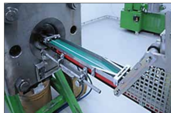
Fig. 2: Press extrusion at Fraunhofer ICT enabling the processing of small batch sizes for gun propellant development and characterisation as well as the supply of extensive campaigns for performance evaluation
