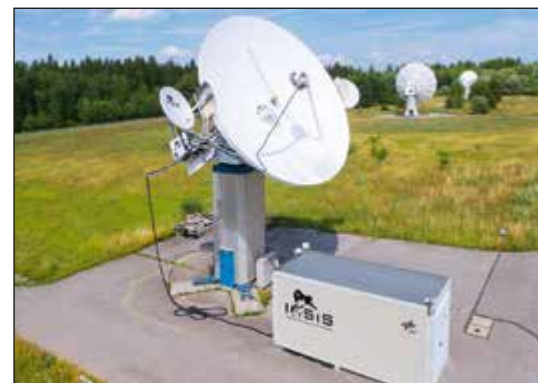
Fig. 1: IoSiS radar system at DLR facilities in Weilheim, Upper Bavaria. The medium-sized antenna is used for transmitting, the two laterally arranged small antennas for receiving
