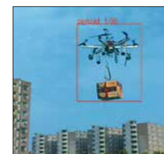
Fig. 5: Recognition of payloads makes it possible to assess danger and thus to prioritise counteraction when detecting a drone swarm
