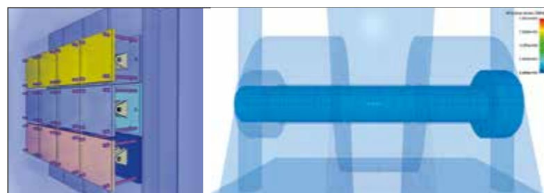
Fig. 2: FEM model of the whole test frame (left) and, as an example, the screw connection M16 not prestressed (right)
