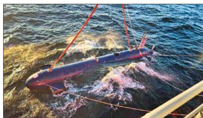
Fig. 1: The LUUV “Blue Whale” being lowered from the accompanying ship for tests
