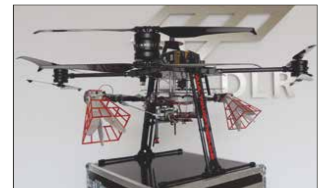
Fig. 4: R&D-demonstrator of a UAV-borne ground penetrating radar system for explosive ordnance detection
