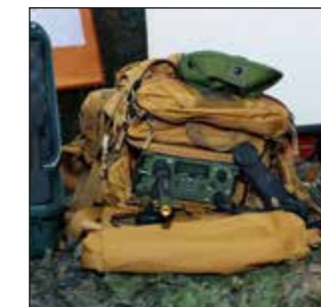
Fig. 6: AN/PRC 160 ManPack; transmission medium within the CD&E project
