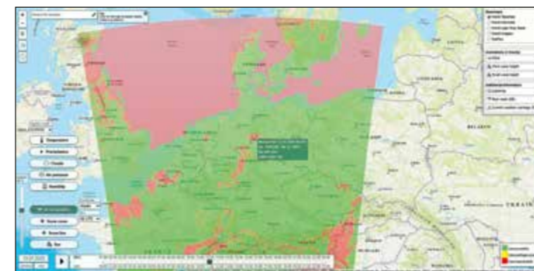
Fig. 3: The webservice. Presented is a traffic light forecast depending on the drone type, which states if the weather situation is expected to be favourable for drone flights. It is possible to choose the drone type, the point of time as well as the numerical weather prediction models for Europe (ICON-EU) or the one for Germany (ICON-D2), both operated by DWD (source: ZGeoBw)
