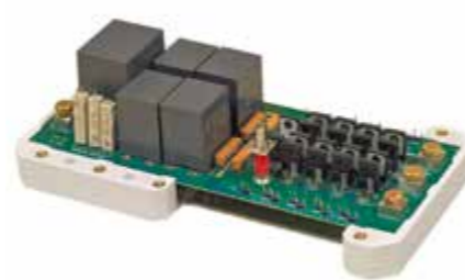
Fig. 3: Power inverter prototype for a 250-kW-capacitor charger
