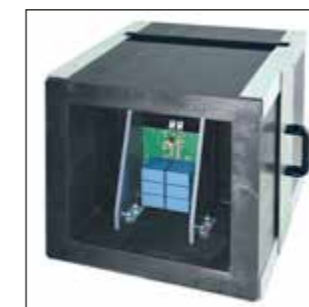
Fig. 4: Shielding box for selective neutron irradiation
