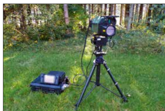
Fig. 1: MILOS-D test sample consisting of laser effector, pan / tilt unit, tripod, laser source, battery and tablet
