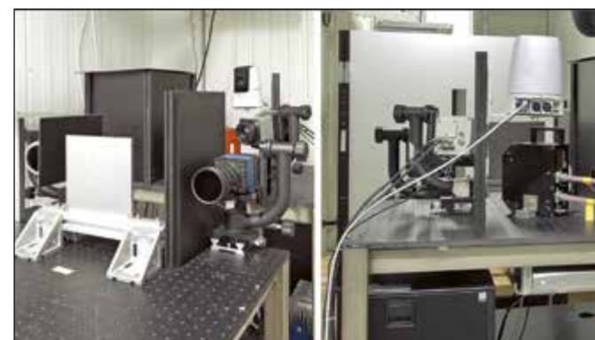
Fig. 1: HEL interaction laboratory, left: target zone with sensors and cameras; right: rear view, scattering screen in the background (distance screen to target zone 1 m)
