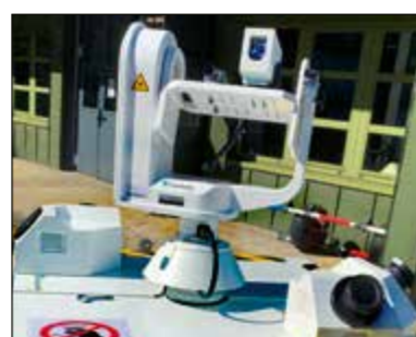
Fig. 3: IOSB experimental system MODEAS for the optical detection, tracking, and analysis of incoming drones
