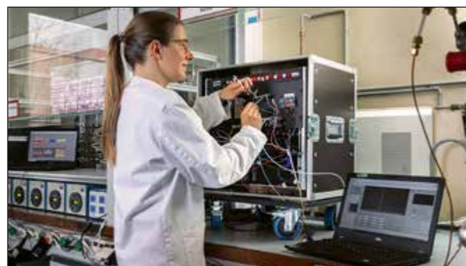
Fig. 1: The HiKE-IMS laboratory prototype was connected to a gas generation system for an extensive quantitative characterisation with chemical warfare agents
