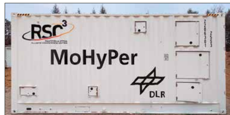
Fig. 1: The Mobile Hydrogen Peroxide Transport and Storage Container „MoHyPer“
