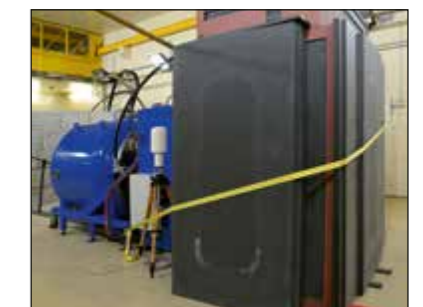
Fig. 6: Neutron beam test chamber at the WIS with shielding
