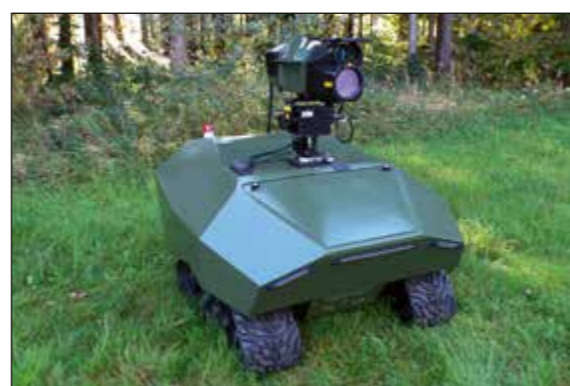
Fig. 2: Laser effector with pan/tilt unit mounted on UGV – Rovo self-propelled platform
