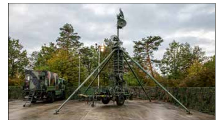
Fig. 4: Terrestrial transmission system (TÜrSys) for long ranges (source: Bundeswehr / Martina Pump)
