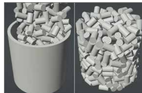
Fig. 2: Filling process of a generic loading space (left) and resulting powder bed (right)
