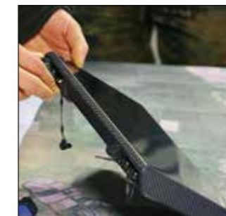
Fig. 4: BACKBONE® model (MUSE), change of security domain by exchanging dongle
