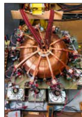
Fig. 2: XRAM – inductive pulsed generator for railguns
