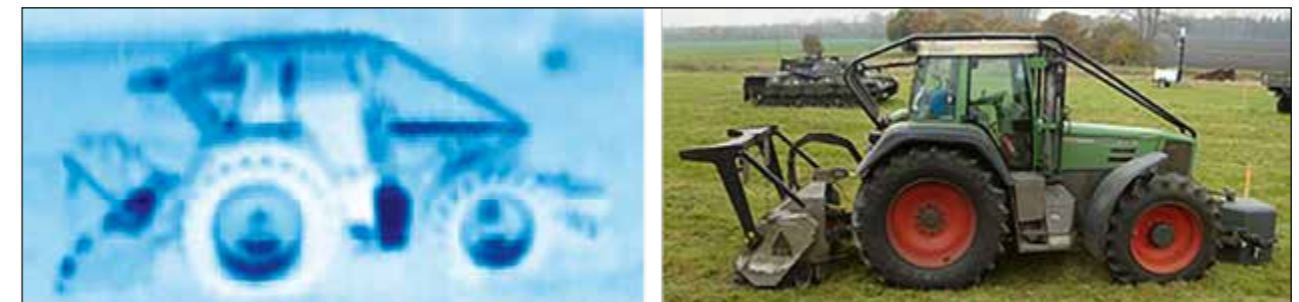
Fig. 3: Example of radiometric imaging in the 80-100 GHz frequency range using conventional scanner and receiver technology (left). Rydberg sensors could be used here to significantly increase performance. Radiometric images are similar to optical images in terms of interpretability (right) and are also possible in poor visibility conditions
