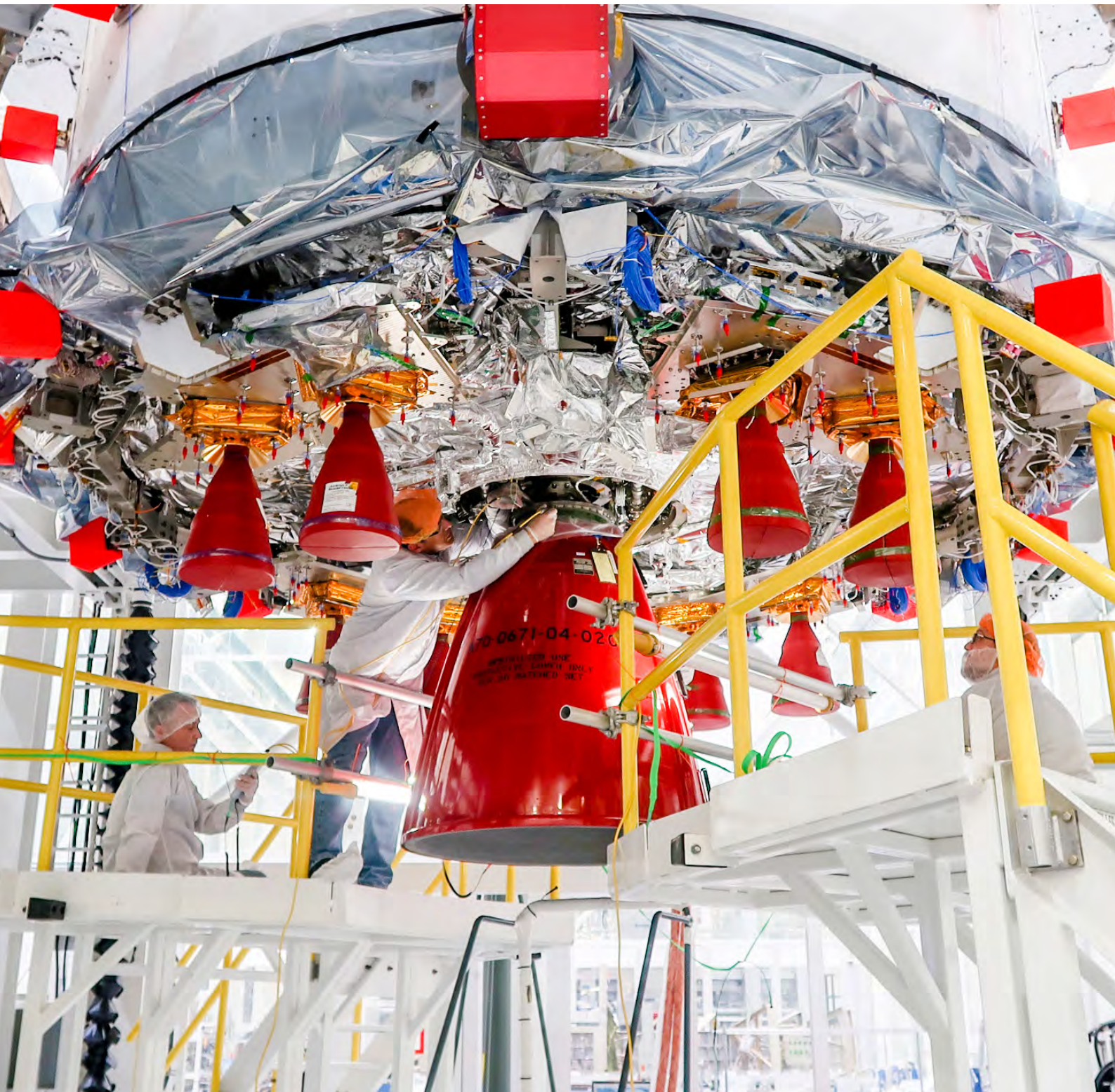
Manufacturing of the European Service Module in Bremen, Germany.
