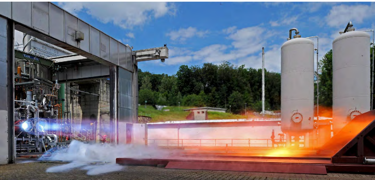
A LOX-methane technology demonstrator is being tested on a test bench.
