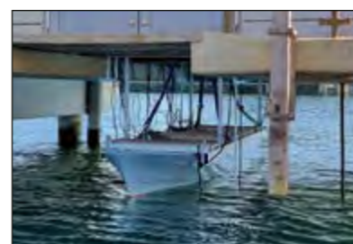
Fig. 3: Fast attack craft model tied up underneath the WTD 71 measuring station in Lake Ploen
