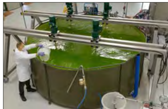
Fig. 2: Organic test water in a basin with agitator
