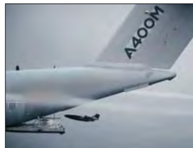
Fig. 1: Example of a remote carrier being dropped from a military transport aircraft. This shows the launch of a DT25 from the A400M, which was carried out as part of the UAV Launcher project initiated by Airbus (Source: Airbus)
