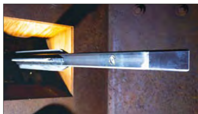
Fig. 2: Pressure lance for incident blast pressure measurement
