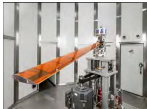
Fig. 1: Investigation of an active twist rotor blade in a whirl tower
