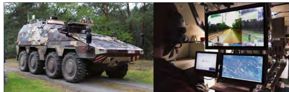
Fig. 1: Left: Joint Operational Demonstrator for Advanced Applications (JODAA). Right: Interior view with augmented reality overlays in the camera-monitor vision system, developed by Fraunhofer FKIE
