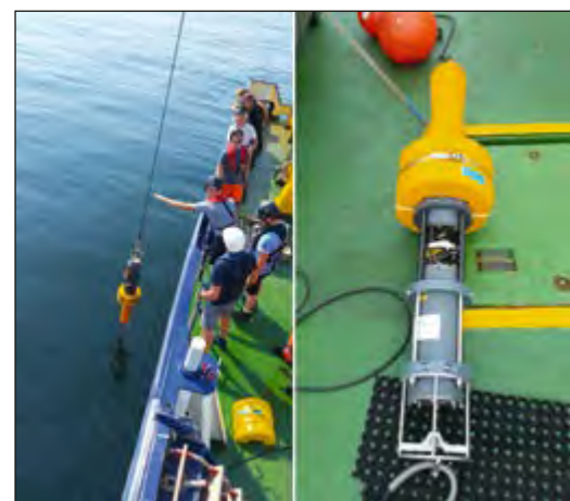
Fig. 1: Recording buoy, produced by Jasco Applied Sciences Ltd., with single hydrophone (right); deployment of buoy from research vessel ELISABETH MANN BORGESE (left)
