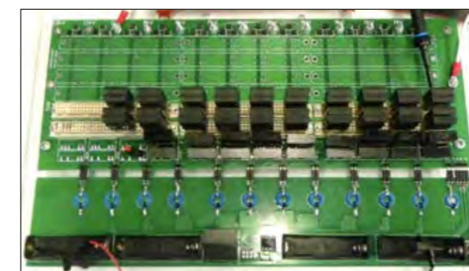
Fig. 4: Test board for studying SiC-MOSFET switching arrays, here equipped with 40 SiC MOSFETs in a (10 x 4)-array
