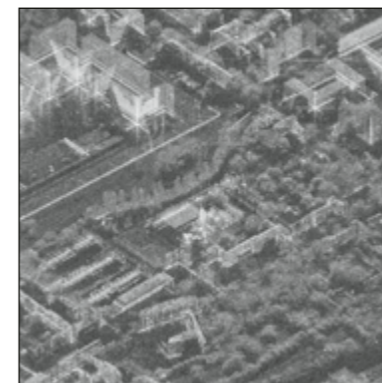
Fig. 4: SAR signature (TerraSAR-X) of a chimney that can hardly be seen due to SAR-specific imaging effects (Berlin, August 2017)
