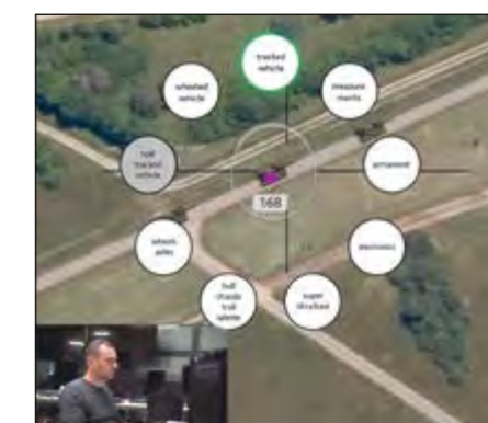
Fig. 4: Recognition assistance with AI-based voice input: The recognition features arranged around the target object can be entered into the system for target object determination by means of voice commands while keeping the visual attention on the target object
