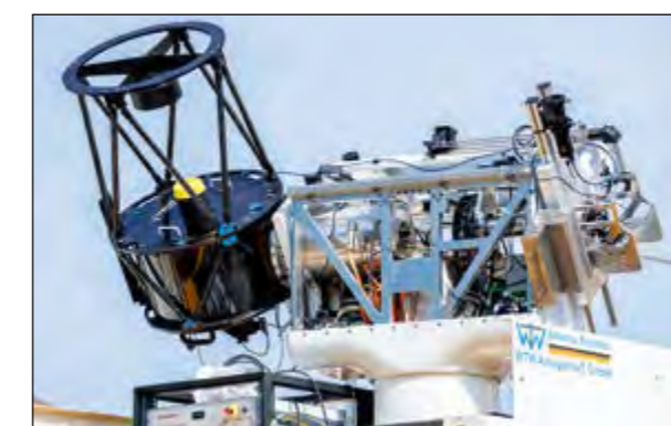
Fig. 4: Telescope mount with receiving telescope (left) and transmitting telescope (right) on the lifting platform of the containerised ground station (STAR-C: Surveillance, Tracking and Ranging Container)
