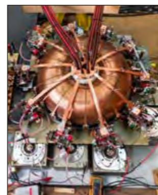
Fig. 3: XRAM generator – inductive pulsed power generator for railguns
