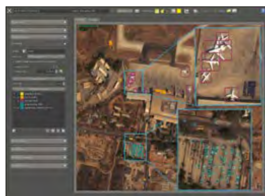
Fig. 1: AI-based object detection in the ABUL video exploitation system. The imagery shows the detection of aircraft, passenger cars and trucks (image section: XView, cf. Lam, Darius, et al. "xview: Objects in context in overhead imagery." arXiv preprint arXiv:1802.0785 (2018))
