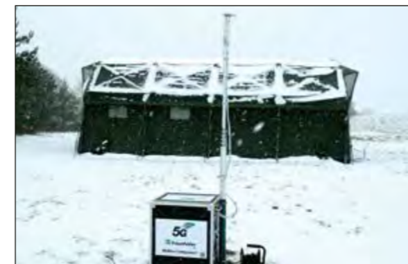
Fig. 3: Setup for measuring the influence of an inflatable tent for command posts on 5G communications
