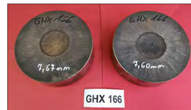
Fig. 3: Results from plate dent testing
