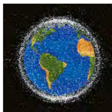
Fig. 1: Current representation of catalogued objects in low Earth orbit (Source: NASA Orbital Debris Program Office)
