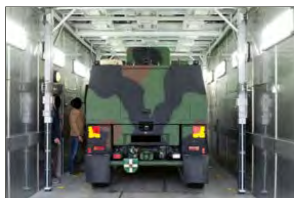
Fig. 1: Examination of the EAGLE V in the climate chamber at WTD 41
