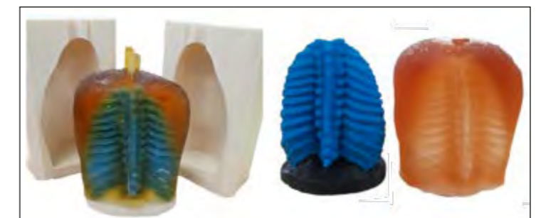
Fig. 4: Casting mould with core, made by additive manufacturing for creating the soft tissue
