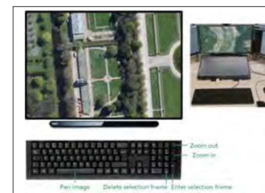
Fig. 3: Experimental system equipped with a Tobii 4C eye tracker below the video exploitation monitor. The pointing operation is accomplished using gaze and allows, for example, selecting the position of relevant objects (e. g. vehicles). Object marking as well as zooming and shifting of images are actuated at the gaze position using various keys of the computer keyboard
