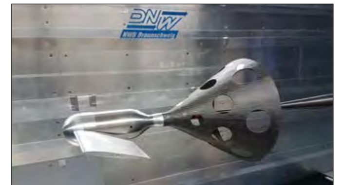
Fig. 4: Wind tunnel measurements on the scaled, controllable refuelling drogue
