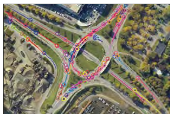
Fig. 2: AI-based multi-object tracking in wide area motion imagery (WAMI) showing automatically recognised trajectories for moving vehicles (WAMI image section: Hensoldt, cf. Sommer, Lars, Wolfgang Krüger, and Michael Teutsch. "Appearance and motion-based persistent multiple object tracking in wide area motion imagery." Proceedings of the IEEE/CVF International Conference on Computer Vision. 2021)
