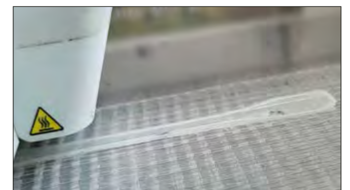
Fig. 4: Creation of a tensile specimen of UHMWPE using FFF
