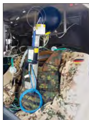
Fig. 2: Dummies developed to simulate the heat and moisture emitted by vehicle crews alongside the measurement technology for recording WBGT values
