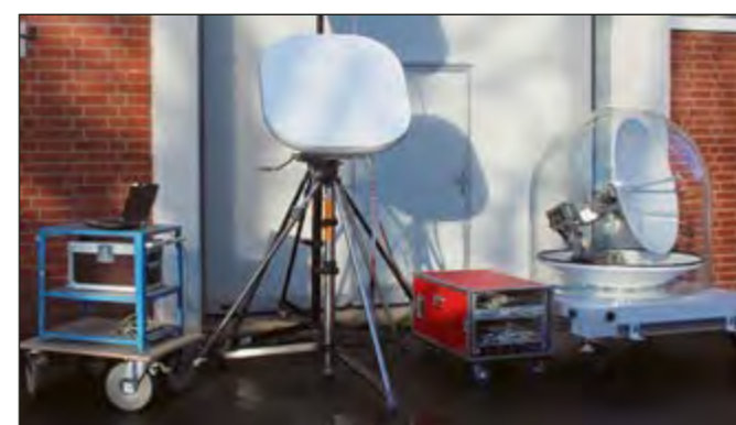
Fig. 2: SABBIA 2.0 passive radar demonstrator with commercial antennas from EPAK (right) and Kymeta (left)
