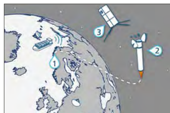
Fig. 1: Concept of operations for OTTER : 1) Launch of ISAR Aerospace Spectrum Rocket from Andøya, Norway 2) Separation in low, elliptical orbit 250 km – 350 km 3) Recording of AIS signals and optical images from ships
