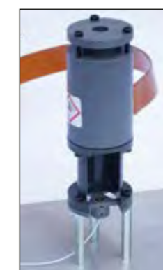
Fig. 4: Experimental setup for combined measurements of detonation velocity and detonation pressure
