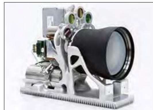
Fig. 2: Main payload: a special camera with a filter wheel as an infrared imager
