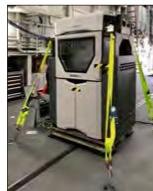
Fig. 2: CD&E experiment frigate SACHSEN: integration of a Level 2 material extrusion printer
