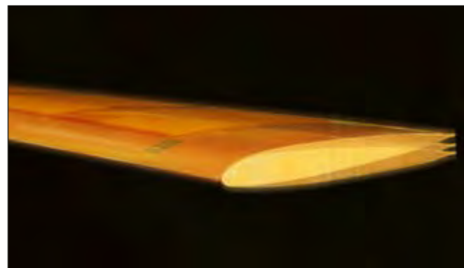
Fig. 2: Blade tip movement of an active twist rotor blade
