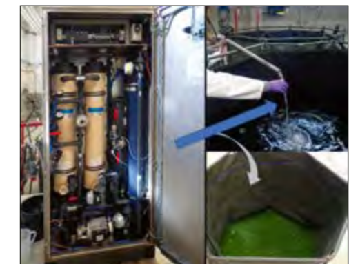
Fig. 4: Backwashable plant during testing with organic test water with clear filtrate and backwash basin
