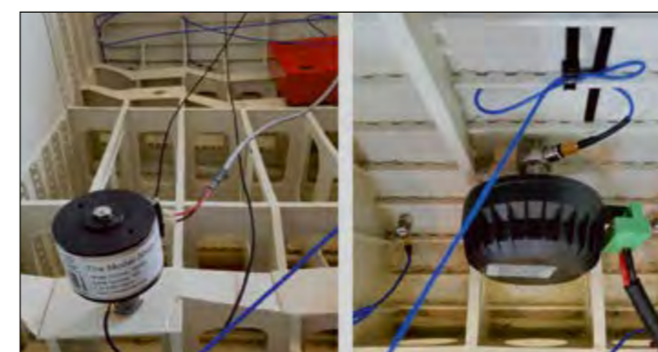
Fig. 4: Inertial actuator in the fast attack craft model to generate the actual signature (left) and inertial actuator and accelerometers on the hull shell to generate the desired target signature (right)
