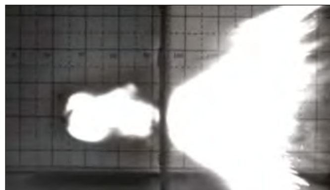
Fig. 1: Perforation of an armour steel plate by a surrogate fragment from left to right, obtained with high-speed imaging. The energy release and expanding reaction zone after perforation are shown clearly
