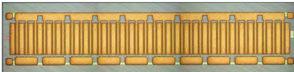
Fig. 1: Micrograph of a 100 V GaN transistor with an output power of more than 400 W at S-band frequencies (2 – 4 GHz)
