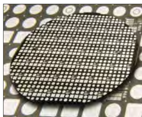
Fig. 1: 100-mm epi-wafer comprising SiC thyristor devices with varying dimensions
