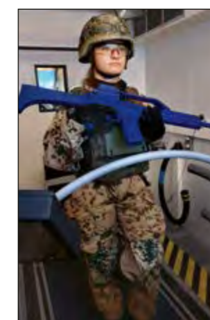
Fig. 4: Test subject during the test inside the climate chamber to investigate the effectiveness of the body cooling vest
