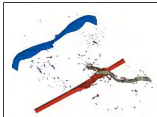
Fig. 2: Numerical simulation of an ERA against an APFSDS projectile
