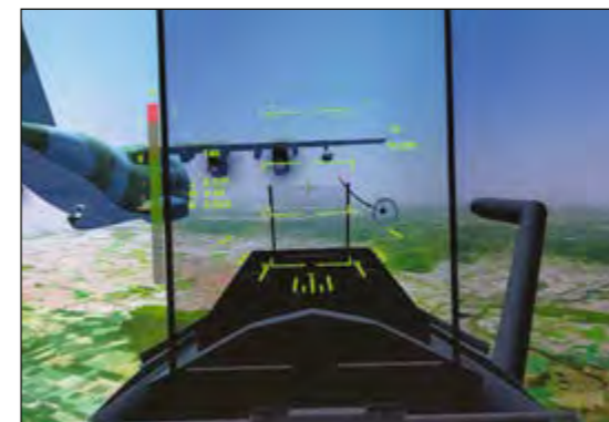
Fig. 3: Test of an assistance system for air-to-air refuelling of combat aircraft using the Microsoft HoloLens
