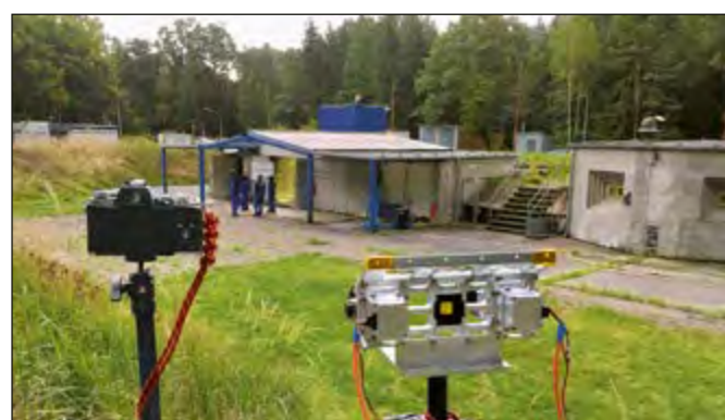
Fig. 1: View of the test stand with cameras for the visual (left) and infrared spectrum (right) in the foreground
