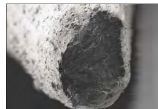
Fig. 3: Fracture surface of a filament made of UHMWPE with increased strength (SEM image, voltage 0.805 kV, working distance 2.1 mm)
