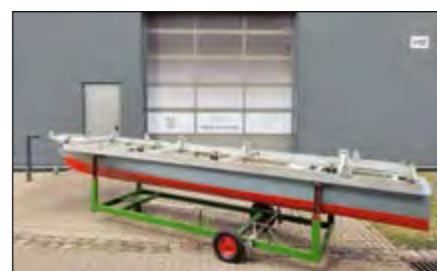
Fig. 2: Fast attack craft model at a 1:8 scale measuring approx. 6 m in length
