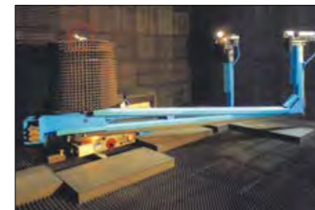
Fig. 3: Measuring facility for the experimental determination of the bistatic radar cross section (RCS), measuring frequency range: 75 to 110 GHz. The device to be measured (scaled aircraft) is highlighted by a red circle
