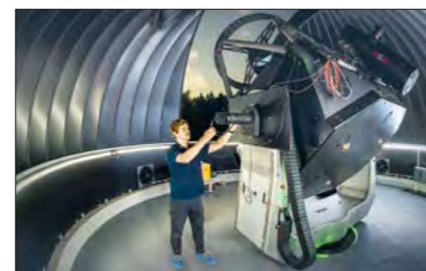
Fig. 3: Reflecting telescope and mount inside the dome of the Johannes Kepler Observatory
